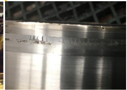
Magnetic solids found in back of primary ring
