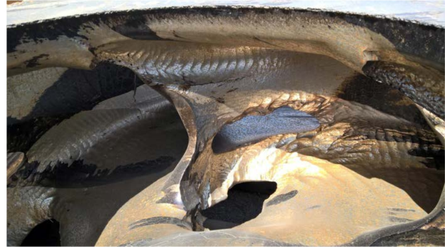
Leading edge and back shroud became weak points - The “Supertanker” design will be implemented and is expected to help reducing local wear
